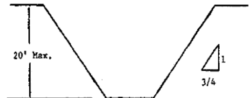
Figure 45: Section View of Excavation of Soil Class A (image provided by OSHA)
